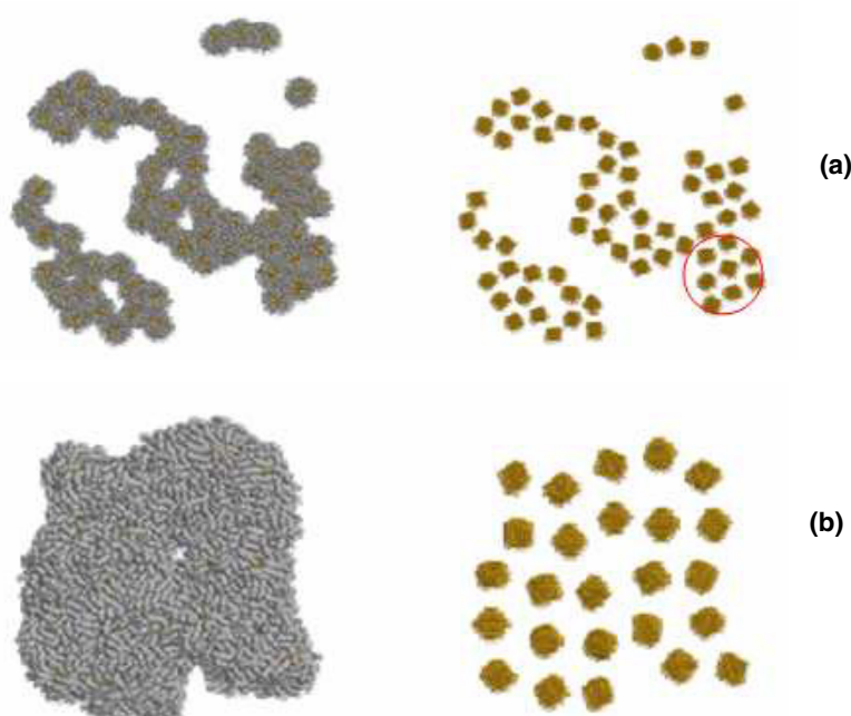
Figure 9. (a) Two-dimensional array of butanethiol nanoparticles. Figures represent the array with (left) and without (right) the passivating layer. The formation of hexagonal lattice has been highlighted. (b) Array of dodecanethiol nanoparticles [90].
